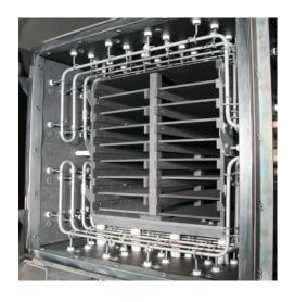
Additionally, 6 zone temperature control front, middle, and rear, for the top and bottom around the retort.
